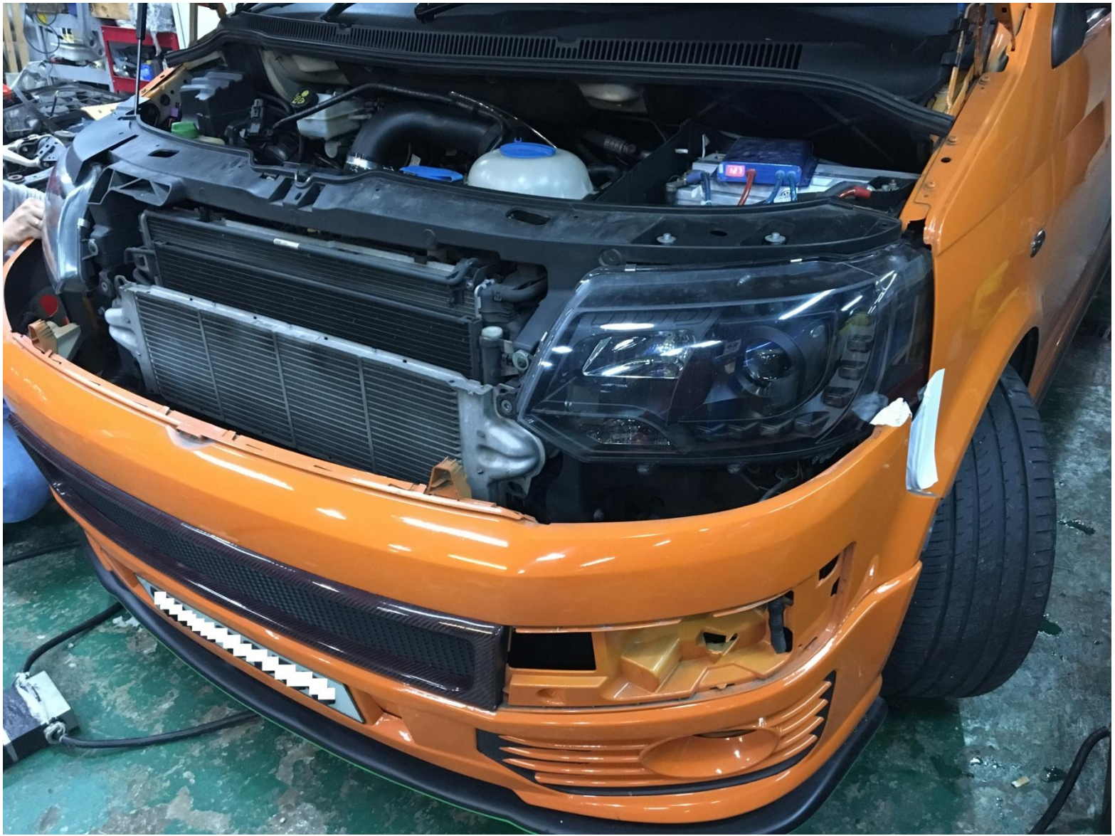
Front grille is removed ready for the dyno of the standard intercooler
