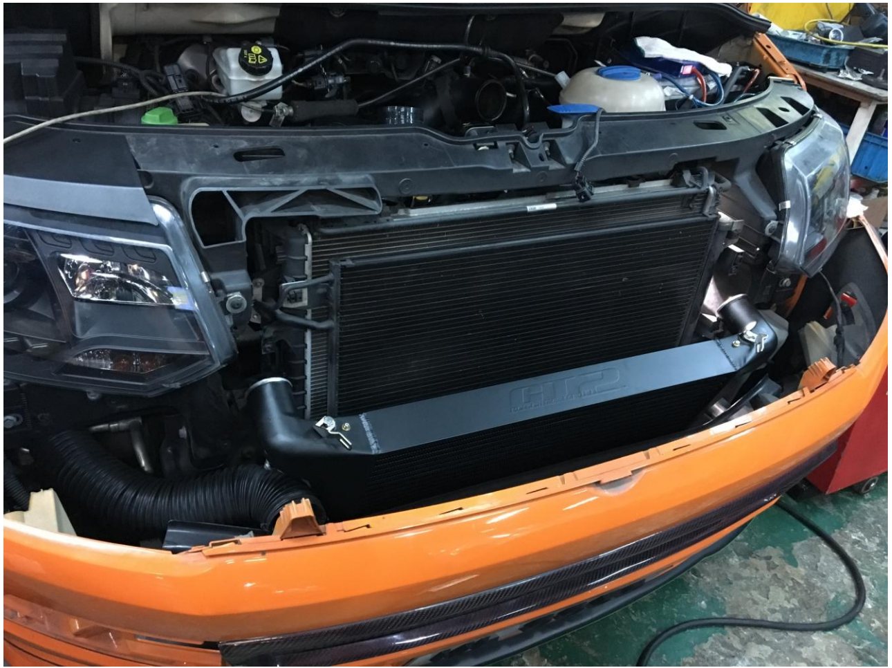
The HDi silicon hoses can also preinstalled while the HDi intercooler positioned as shown.
