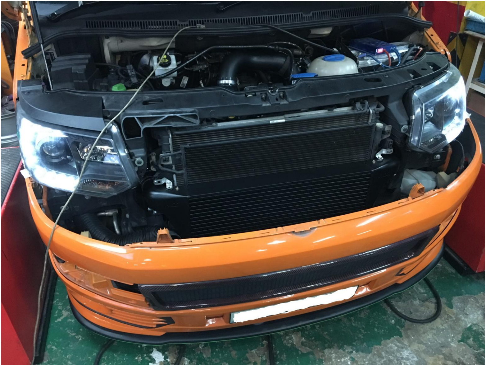
Test with the HDi GT2 intercooler kit installed Test completed
